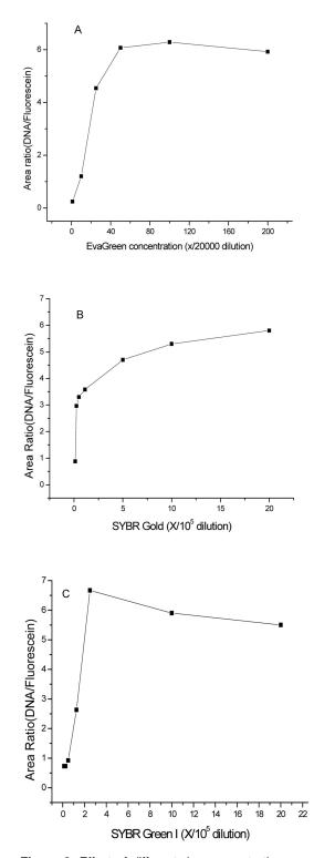
**Figure 2.** Effect of different dye concentrations on fluorescence intensity for  $\lambda$ -Hind III DNA. The  $\lambda$ -Hind III DNA at a total concentration of 240 ng/mL was injected by pressure (0.5 psi, 6 s). Coated capillary (20 cm effective length, 75  $\mu$ m id) was used, filled with 80 mM TAPS solution, containing different concentrations of dyes. Electrophoresis buffer was 80 mM TAPS buffer solution (pH 7.6), the temperature was 25°C, and the applied voltage was -400 V/cm.
