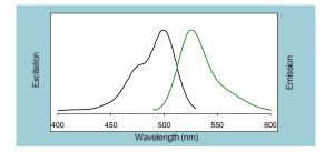
Figure 1. Excitation (left) and emission (right) spectra of EvaGreen<sup>™</sup> dye bound to dsDNA in pH 7.3 PBS buffer.
