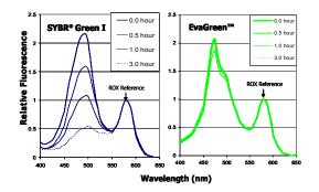
Figure 2. A solution of EvaGreen<sup>™</sup> dye or SYBR<sup>®</sup> Green I each at 1.2 μM in pH 9 Tris buffer was incubated at 99 °C. The absorption spectrum of each solution was followed over a period of 3 hours. ROX was added as a stable reference.
